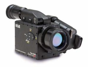
Can detect "Greenhouse Gases" with an estimated atmospheric lifetime of 3,200 years. It can also detect more than 20 other gases in addition to SF6 – ideal for the utility industry and other manufacturing.
