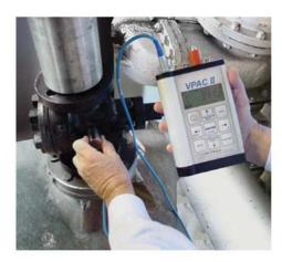
Acoustic Emission (AE) technology has been developed as a solution for this inspection with both manual testing and permanent installations for the purpose of detecting and quantifying the leak rate.
