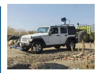
The working principle of this methane gas leak detector is based on a pulsed beam from a diode laser which is directed at the location or area to be inspected.
